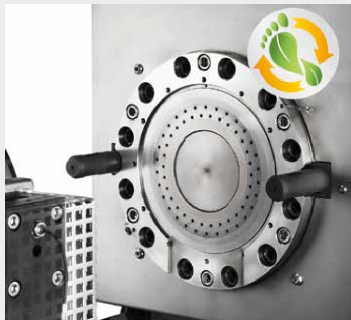
easily accessible die plate unit and hydraulic lock
